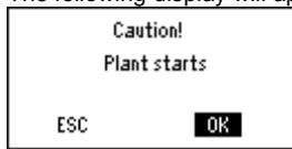
10. Press the select-and-push knob for OK. The application will be started, all sensors will be checked, and sensors used will be monitored further on. The main menu will appear:
