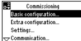
4. Select submenu "Basic configuration". Select the plant type / basic type and the position of the option modules.
